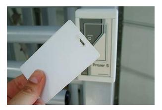
Keyless entry system - Electronic door entry system that has remote control for caretaker to enable users access to hall and room as per agreement (negating the need for issuing keys as users can have a programable card to times and access of hire).
